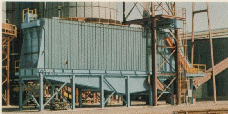
Hinged rear door provides for fast removal of contaminated material or easy access in case of fire.
