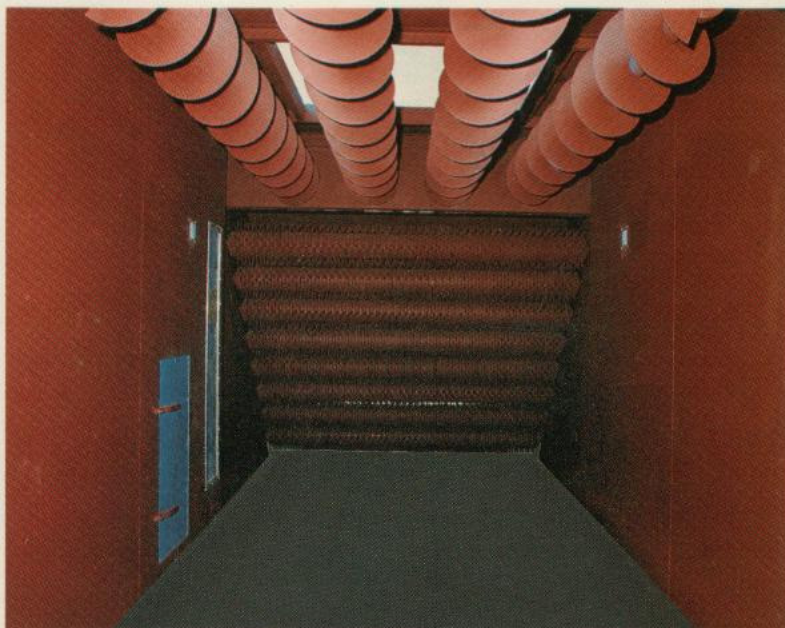
The full width live bottom insures first in first out metered discharge of the material through the doffing rolls.
